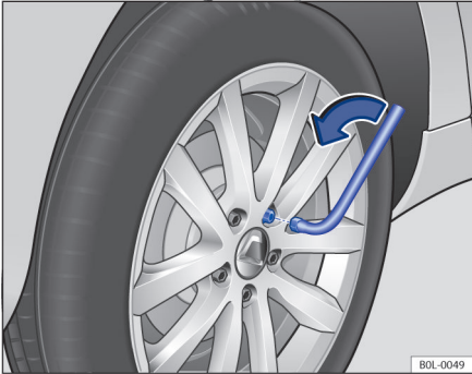
Fig. 157 Wheel change: Unscrew the wheel bolts with the wheel wrench
