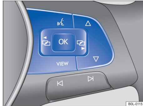
Fig. 17 Right side of multifunction steering wheel: Keys for operating instrument cluster menu and information display (this type is an example only)
