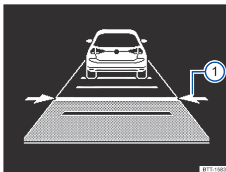
Fig. 97 On the instrument cluster display: set distance (illustration, the ACC is controlling distance).
