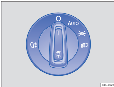
Fig. 65 Beside the steering wheel: Light switch (this type is only an example)
