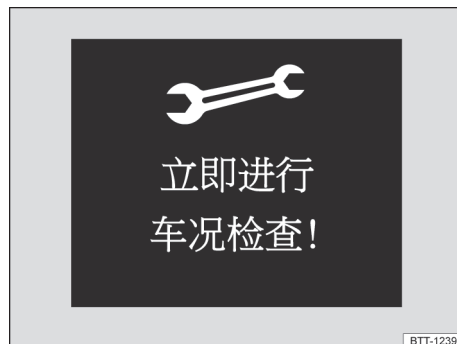
Fig. 16 In the display of the instrument cluster: An example of the display when a maintenance project is due (schematic)
