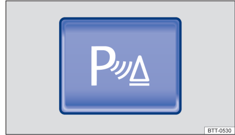
Fig. 100 In the upper section of the centre console: Park Distance Control button (illustration).
