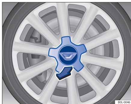
Fig. 151 Removing the centre wheel trim by pulling off
