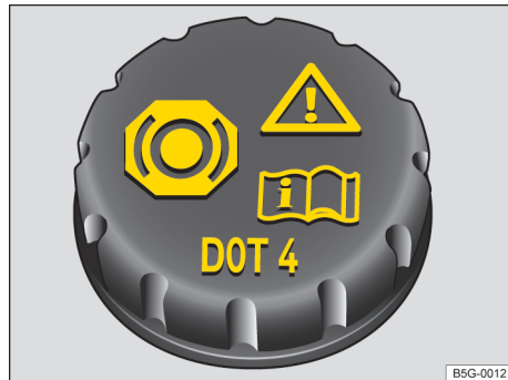
Fig. 140 In the engine compartment: cap of the brake fluid reservoir
