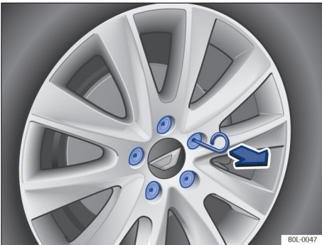
Fig. 150 Removing the wheel bolt caps (illustration)
