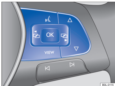
Fig. 19 The right side of the multifunction steering wheel: Keys for the operating instrument cluster menu and information display (this type is an example only)
