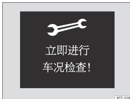
Fig. 18 In the display of the instrument cluster: An example of the display when a maintenance project is due (illustration)
