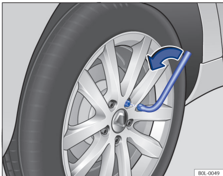
Fig. 155 Wheel change: Unscrew the wheel bolts with the wheel wrench
