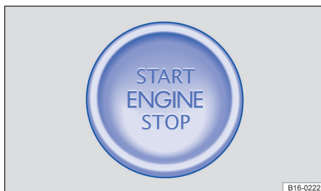
Fig. 83 In the lower section of the centre console: starter button for starting the engine.
