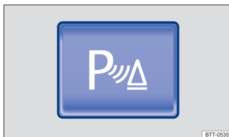
Fig. 100 In the upper section of the centre console: Park Distance Control button (illustration).
