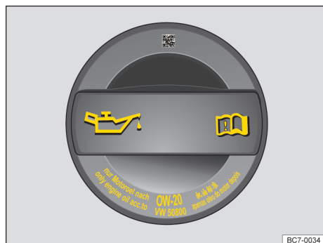
Fig. 135 Sticker showing the engine oil standard (illustration)
